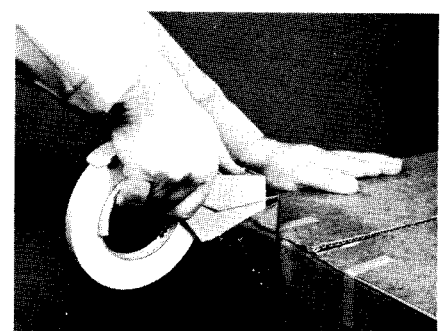
Figure 5 — With brake tension on the tape roll, push the H-131 straight downward to cut the tape and buff it against the box to complete the application.
